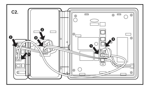
Figure C2: Attaching cable connection of the DHA to an optional button module and the deskphone.
